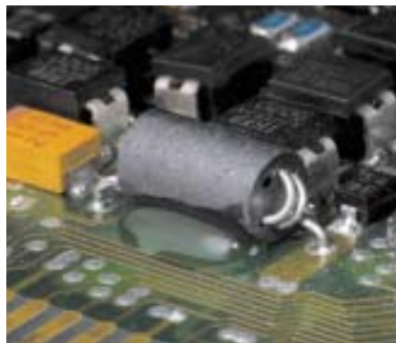
Component rigidization – 3M™ Scotch-Weld™ Epoxy Adhesive DP-125EG reaches handling strength within 3 hours at room temperature. Stabilizes board components with 1500 psi shear strength and 20 piw.
