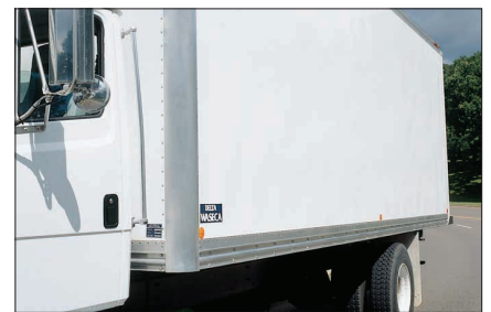
After hundreds of thousands of miles of jarring and bouncing, seams sealed with VHB tape remain securely locked in place. VHB tape absorbs shock, fatigue, and vibration.
